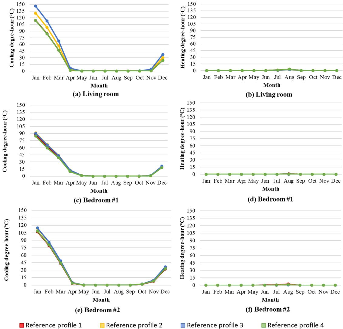
Figure 10 - Annual cooling and heating degree-hours for each room and each reference profile
