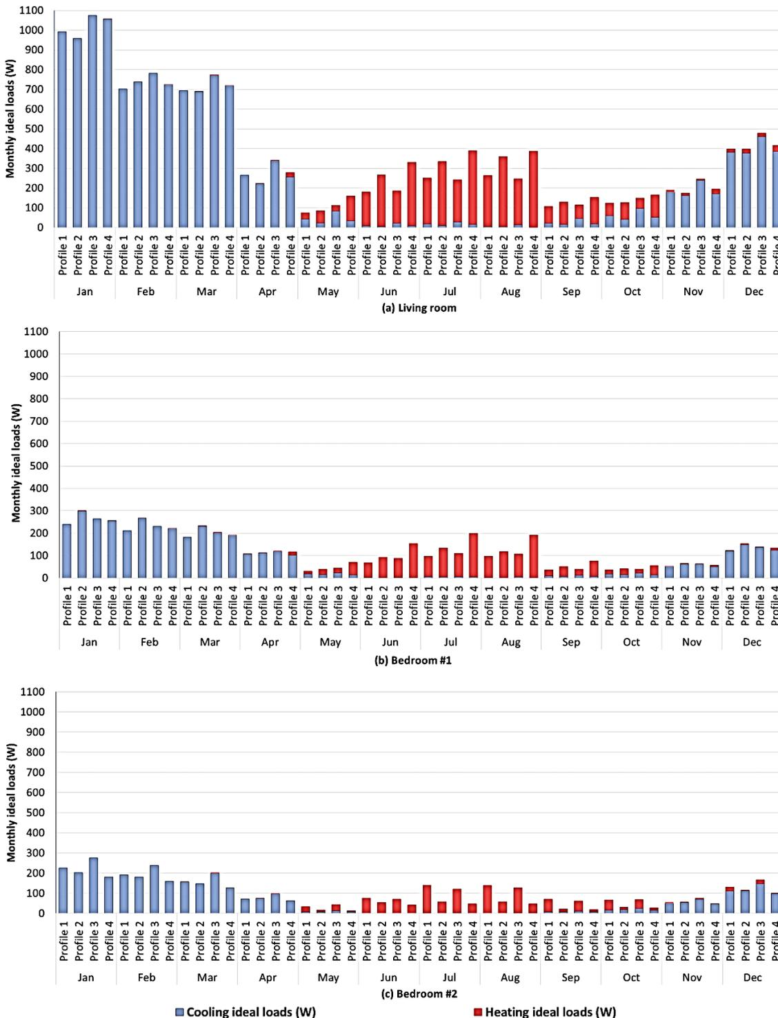
Figure 13 - Annual load for heating and cooling for each reference profile
