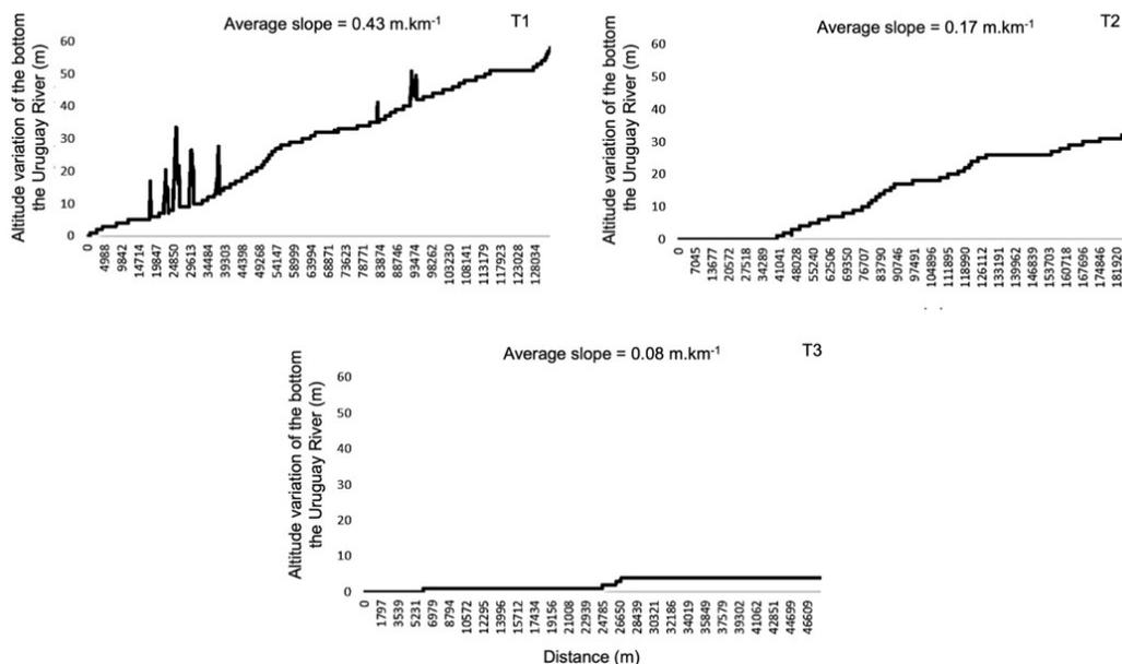
**Figure 3.** Altitude variation of the bottom (m) and the indication of the average slopes ( $m.km^{-1}$ ) of the three sampling stretches of the Uruguay River.
