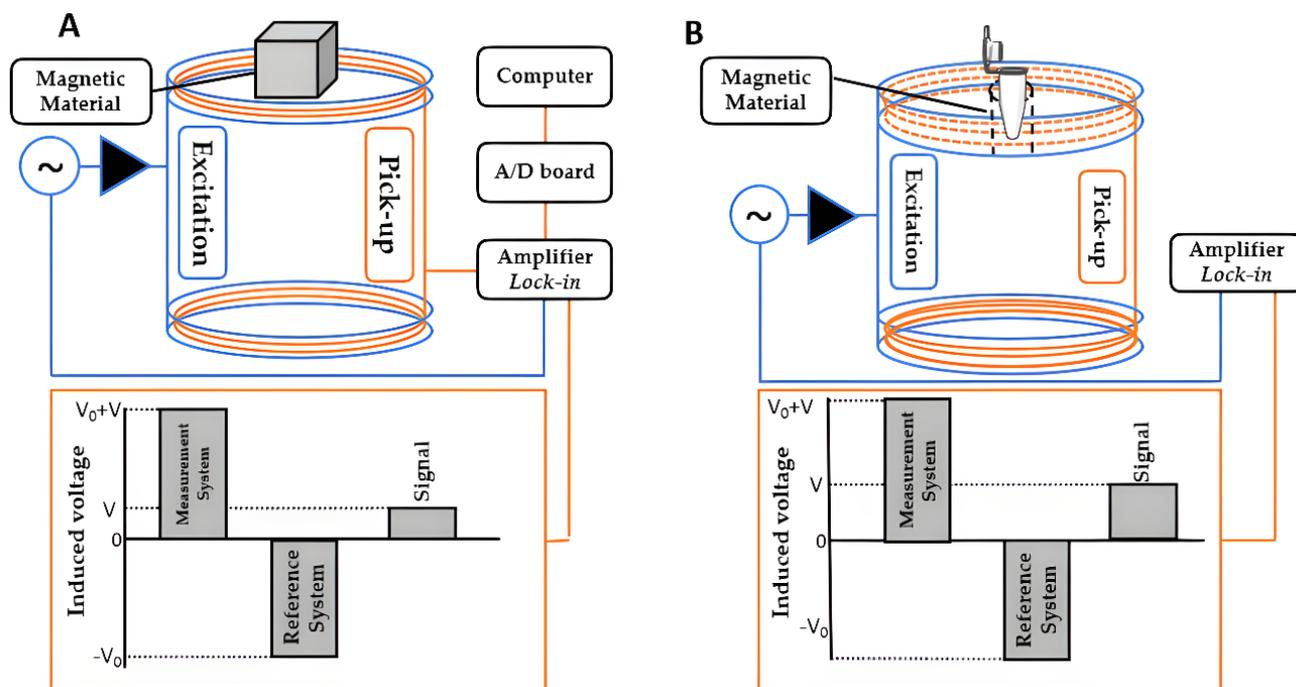
**FIGURE 1** - (A) Schematic diagram of operation the Alternate Current Biosusceptometry (ACB) sensor MonoACB in the presence of magnetic material. (B) Schematic diagram of operation the Alternate Current Biosusceptometry (ACB) sensor Cavity-ACB in the presence of magnetic material. The blue arrows indicate the excitation windings of the coils, and the orange arrows indicate the pick-up windings of the coils.
