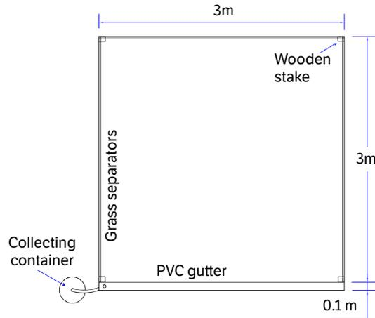
**Figure 1.** Model of collector gutters and their measurements.
