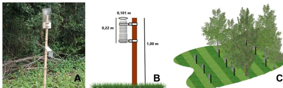
**Figure 3:** Image of the rain collector and installed (A), illustrative scheme of the dimensions of the collector (B), and an illustrative scheme of the collector distribution in the outside, on the edge and in the center of the study areas (C).
