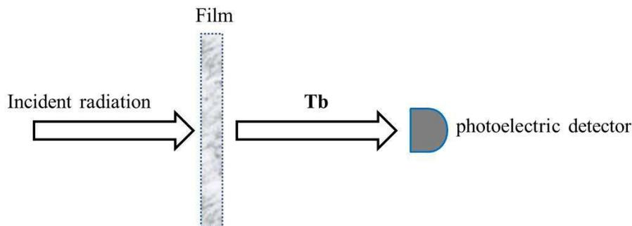
FIGURE. 1 The experimental diagram for transmittance measurement of films. Tb: Ballistic transmittance.
