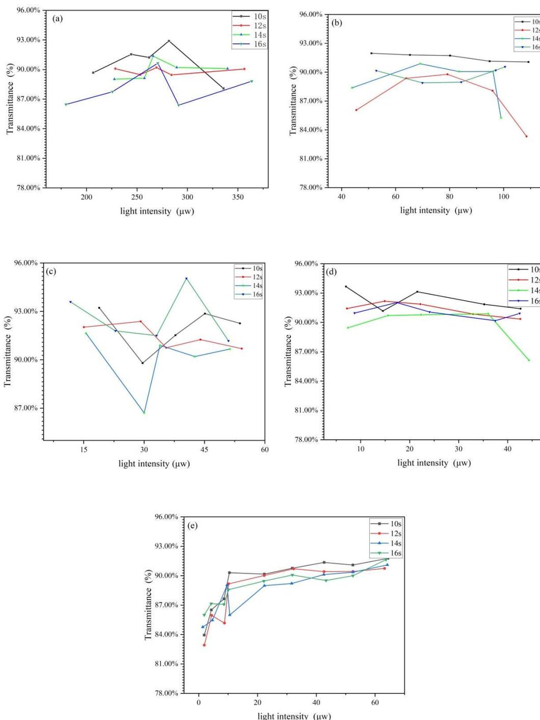
FIGURE 2. The relationships between transmittances and light intensities for several EVA film mulches at different wavelengths. (a): 535nm, (b): 635nm, (c): 830nm, (d): 980nm, (e): 1060nm.
