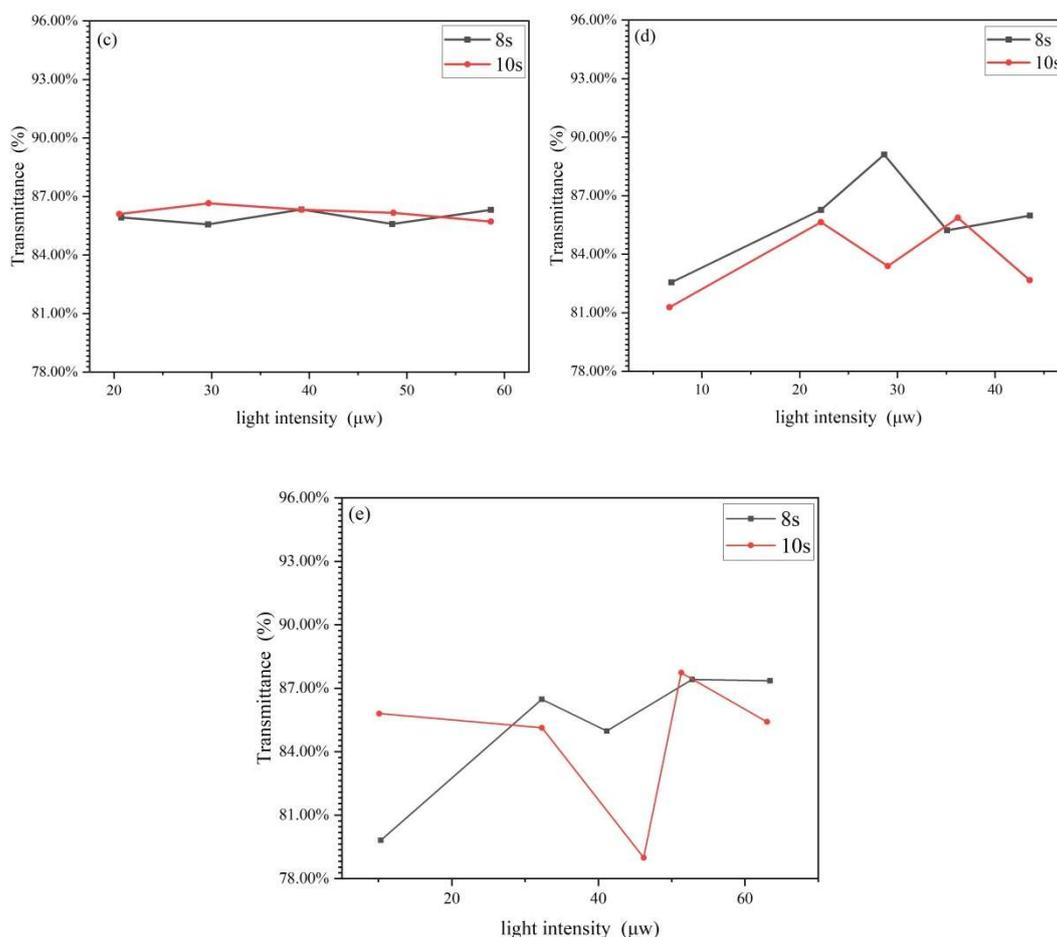
FIGURE 3. The relationships between transmittances and light intensities for two PO film mulches at different wavelengths. (a): 535nm, (b): 635nm, (c): 830nm, (d): 980nm, (e): 1060nm.
