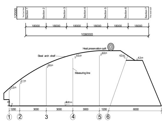
FIGURE 2. Layout of cross section and measuring lines in the greenhouse.
