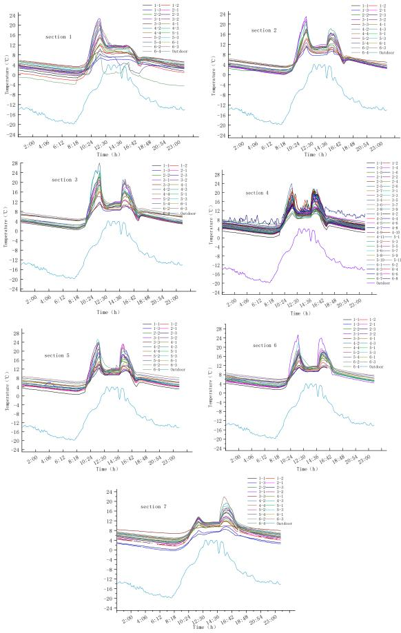
FIGURE 3. Temperature versus time curves for different cross sections (taken on 14<sup>th</sup> January 2020, sunny and snowy the day before, the coldest day of 2020 in Jinzhong, Shanxi Province)
