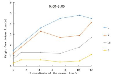
FIGURE 4. Relationships between boundary points of marginal effect and horizontal position during the period 0:00–8:00 on 14<sup>th</sup> January 2019.
