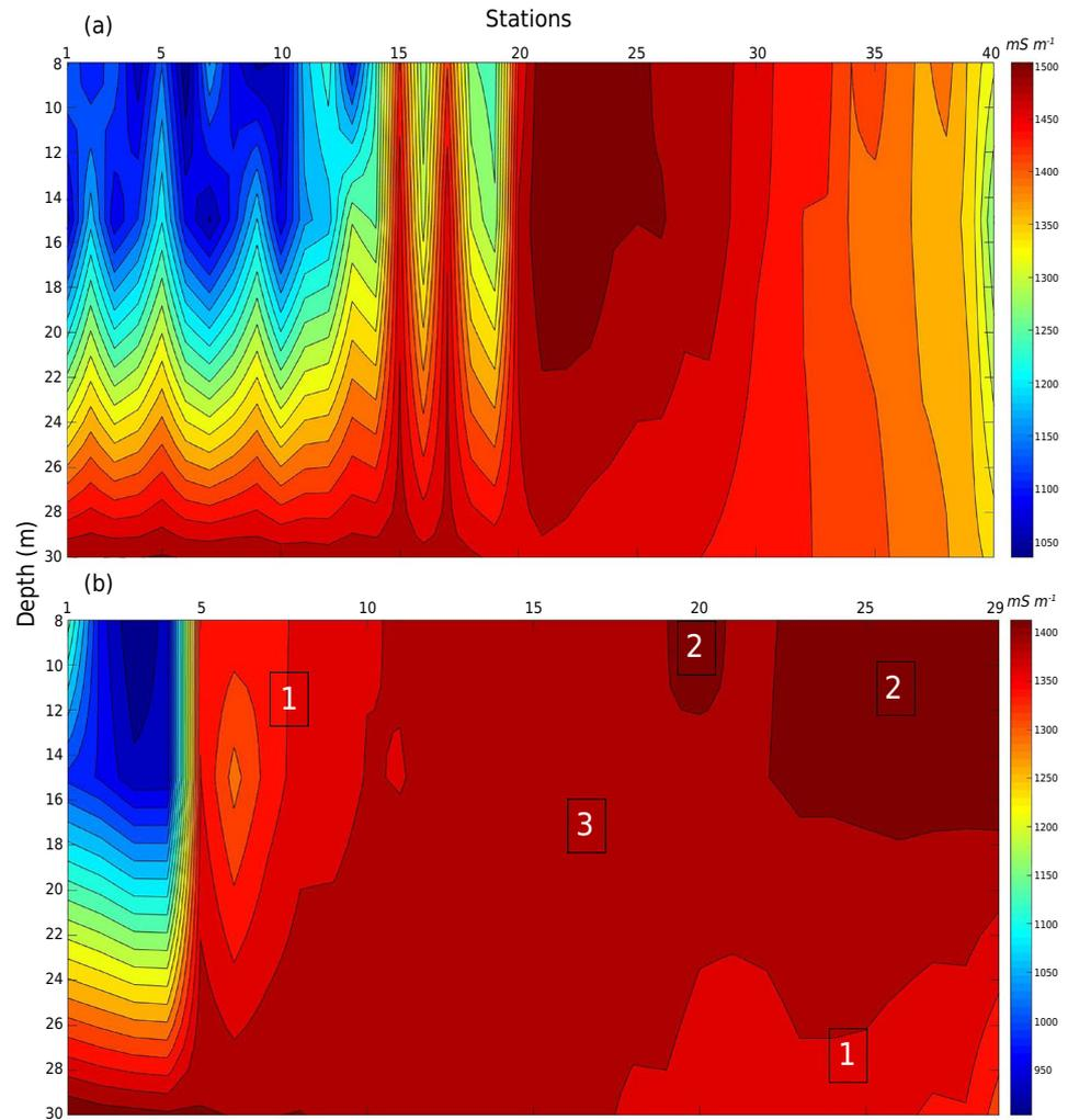
**Figure 6.** Pseudo-sections of apparent conductivity corresponding to (a) profile L1 surveyed during the rainy season (March) of 2021 and (b) profile L2 surveyed during the rainy season (March) of 2021, based on the HD obtained by the cable antenna with coils spaced at 10 m intervals.
