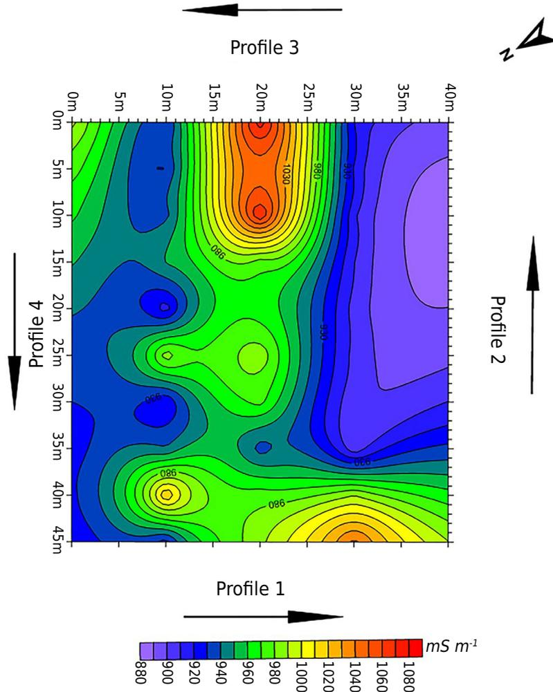
**Figure 4.** Map of apparent conductivity recorded during the dry season (June) of 2021, based on the HD obtained by the cable antenna with coils spaced at 10 m intervals.
