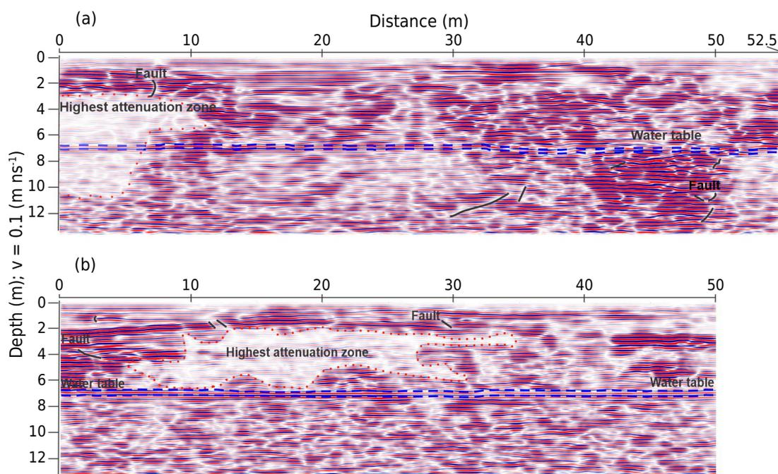
**Figure 3.** FGPR profiles using a 200 MHz antenna (dry season, June 2021): a) profile L3, with a 300 ns time window and b) profile L4, with a 300 ns time window.
