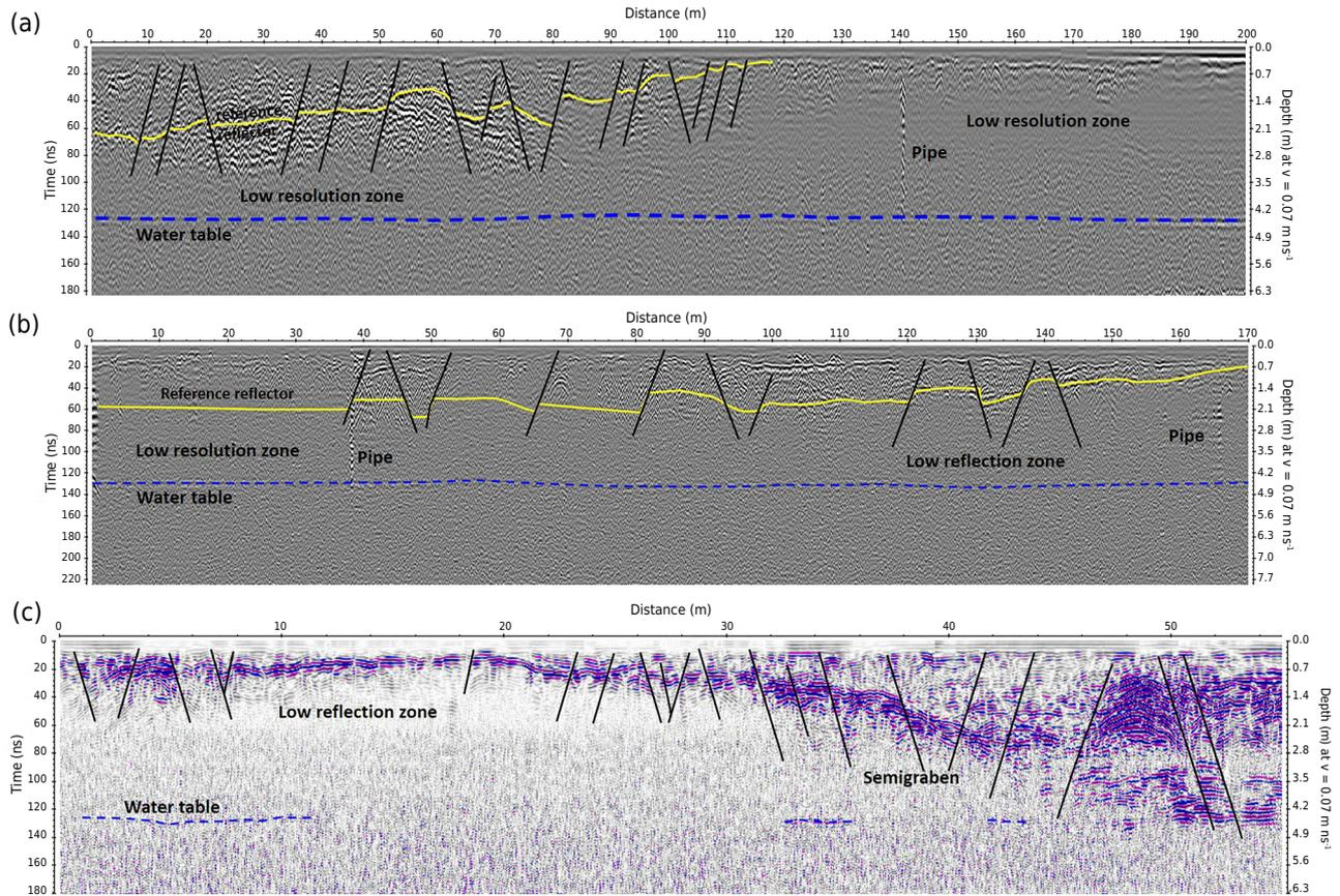
**Figure 5.** The GPR profiles obtained with the 200 MHz antenna: (a) L1 (200 ns range), (b) L2 (250 ns range), and (c) L3 (200 ns range). This survey was conducted in October 2020.
