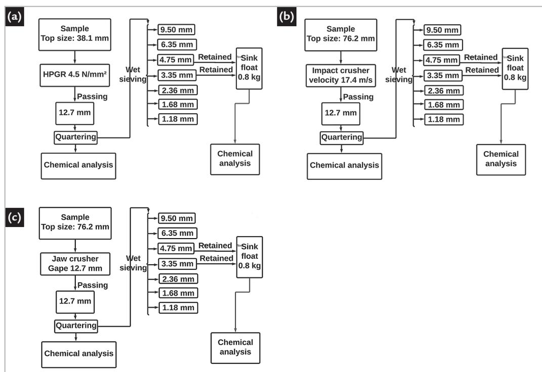
Figure 1 – Test flowchart. HPGR (a), Impact crusher (b), Jaw crusher (c).
