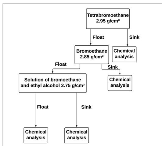
Figure 2 – Sink-float test flowchart.
