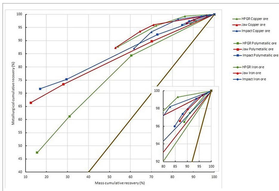
Figure 4 - Metallurgical recovery vs. Mass recovery - fraction - 6.35 + 3.35 mm.
