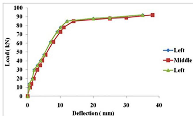
Figure 12: Curve of load versus deflection for beam GB2.
