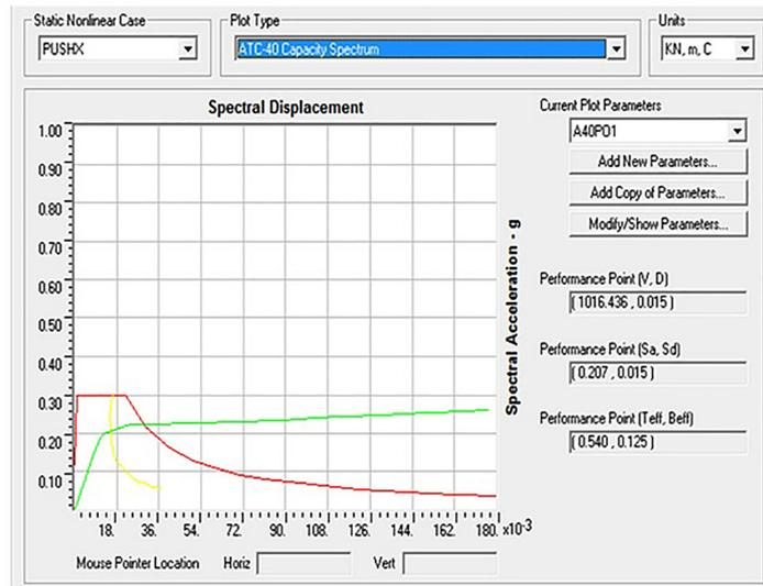
Figure 4: Spectrum of capacity in abscissa.
