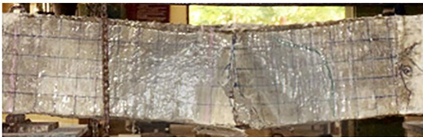
Figure 11: Pattern of beam GB1 failure.
