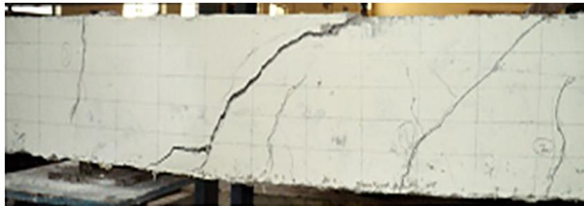
**Figure 9:** Pattern of beam B1a failure.
