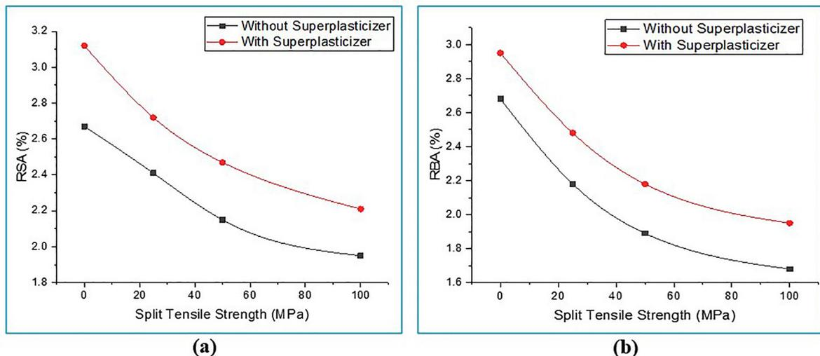
Figure 7: (a) RSAC and (b) RBAC – split tensile strength with/without superplasticizer after 28 days curing period.
