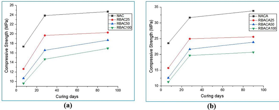
Figure 5: RBAC – compressive strength of cylinder specimens at different curing periods (a) without and (b) with superplasticizer.
