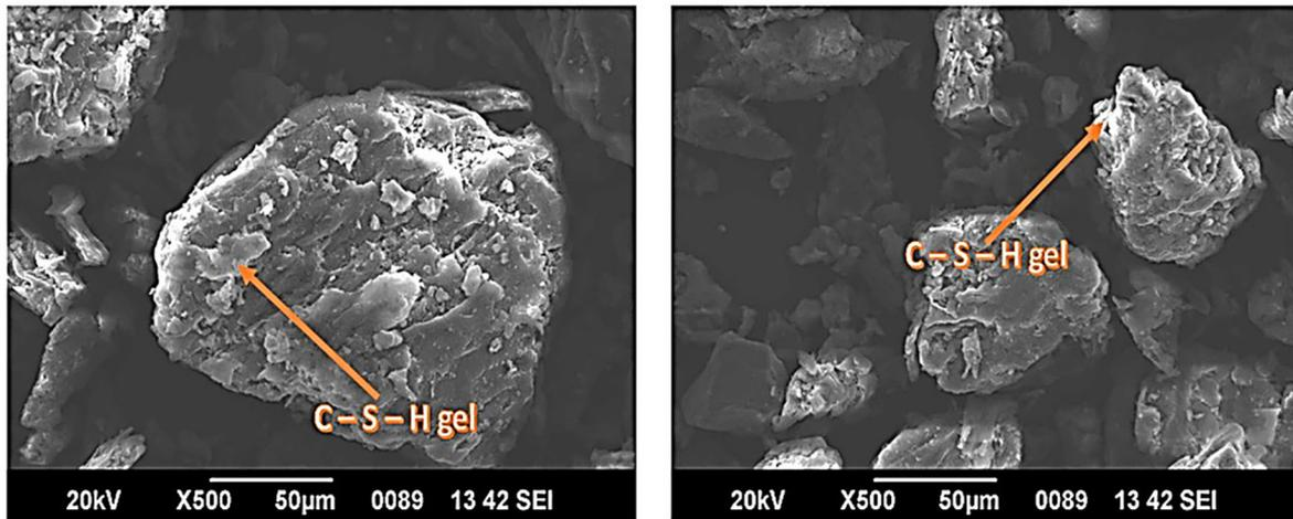
Figure 13: SEM images of (a) RBAC and (b) RSAC concrete mix with superplasticizer.
