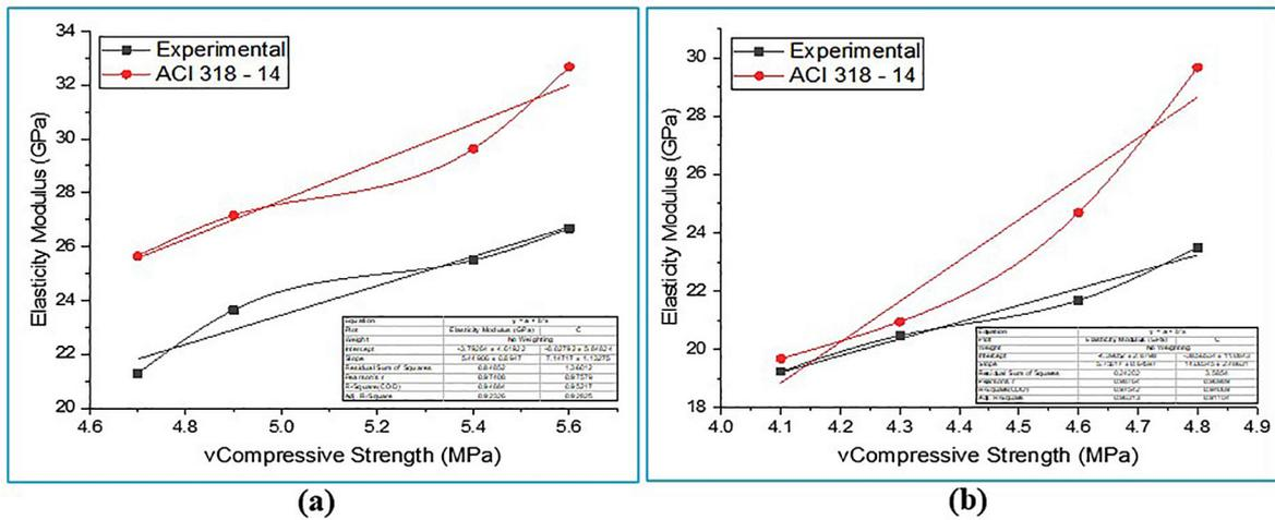
Figure 11: RSAC mixes – elasticity modulus and its relationship with/without superplasticizers.
