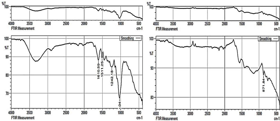
Figure 16: FTIR peaks of (a) RBAC and (b) RSAC concrete mix with superplasticizer.
