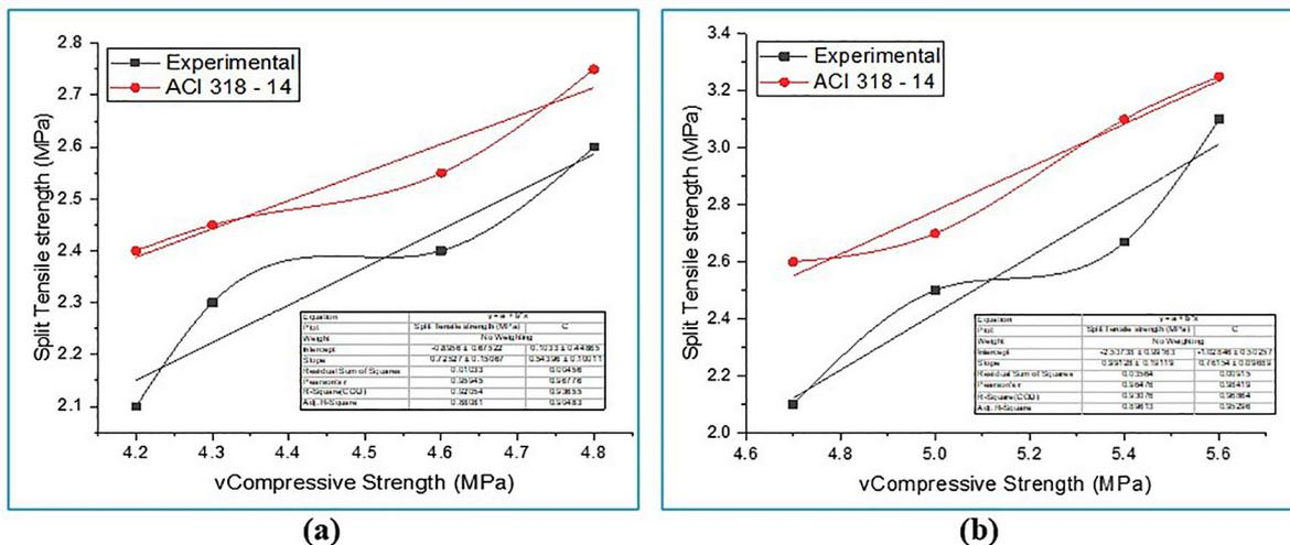
Figure 8: Comparison of the RSAC's split and compression tensile values after 28 days, (a) with and (b) with superplasticizer.
