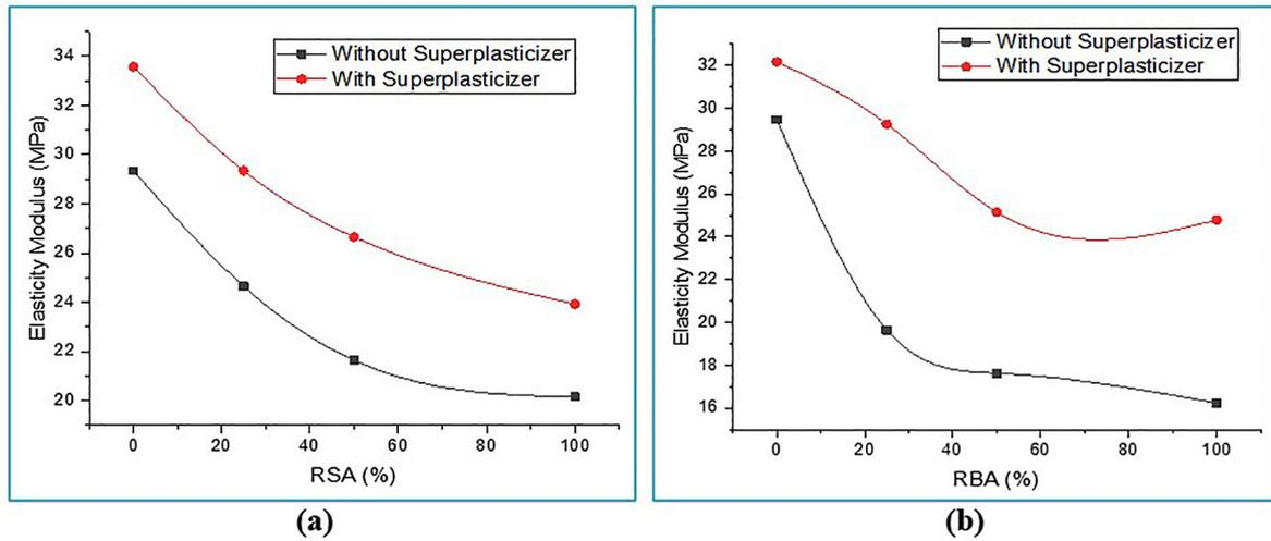
Figure 10: (a) RSAC and (b) RBAC – changes in elasticity modulus and its impact after 28 days of curing time.
