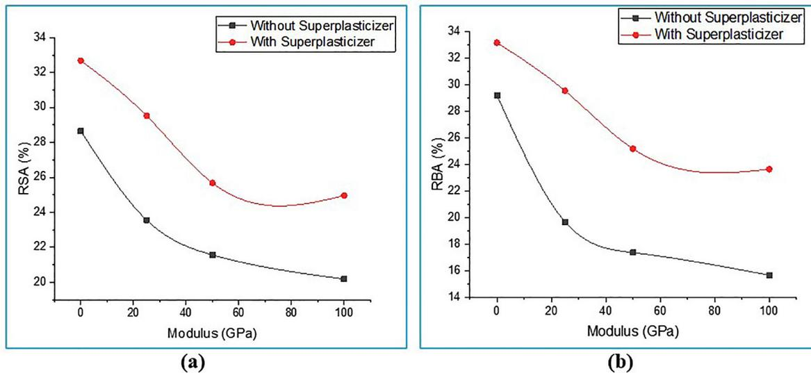
Figure 6: (a) RSAC and (b) RBAC – compressive strength with/without superplasticizer after 28 days of curing period.
