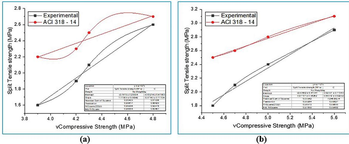
Figure 9: Comparison of the RBAC's split and compression tensile values after 28 days, (a) with and (b) with superplasticizer.
