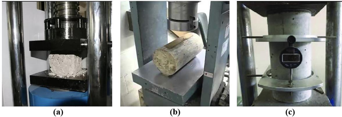
**Figure 3:** Laboratory setup of (a) compression, (b) split tensile and (c) elasticity modulus for concrete mixes.
