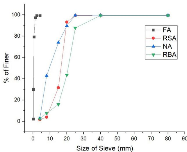
Figure 2: Aggregate types and its size distribution.
