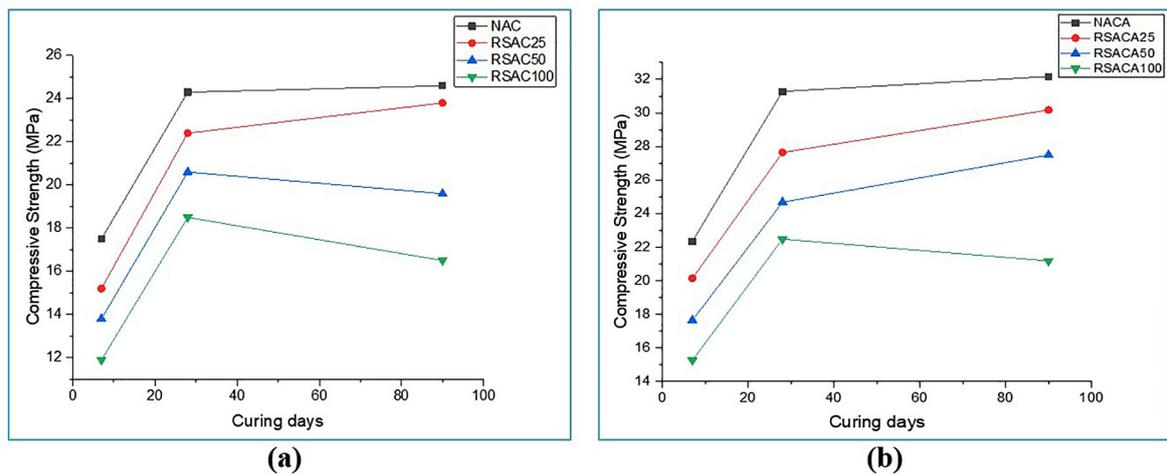
**Figure 4:** RSAC – compressive strength of cylinder specimens at different curing periods (a) without and (b) with superplasticizer.
