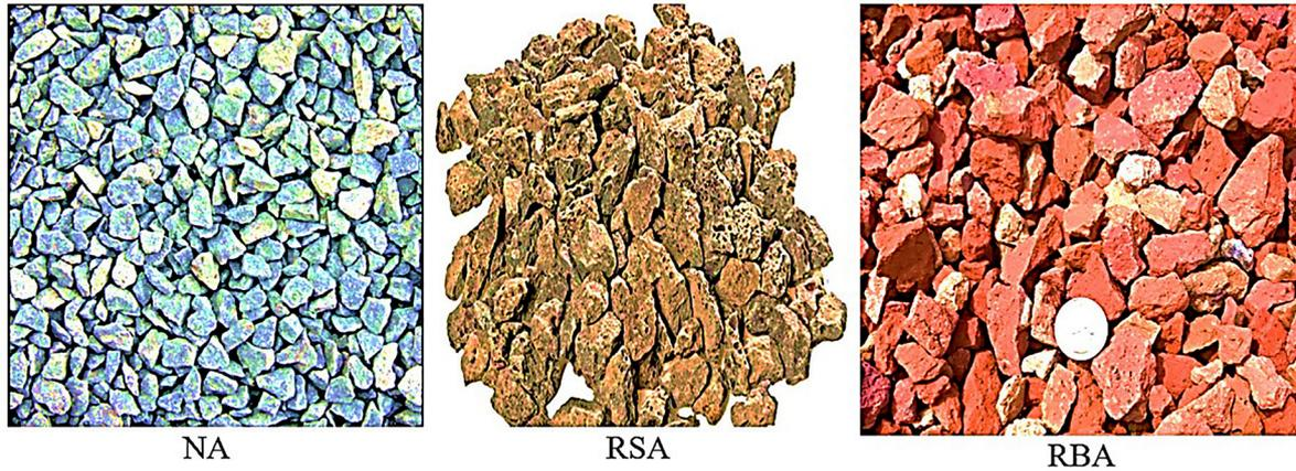
Figure 1: Types of coarse aggregates used for concrete mixes.
