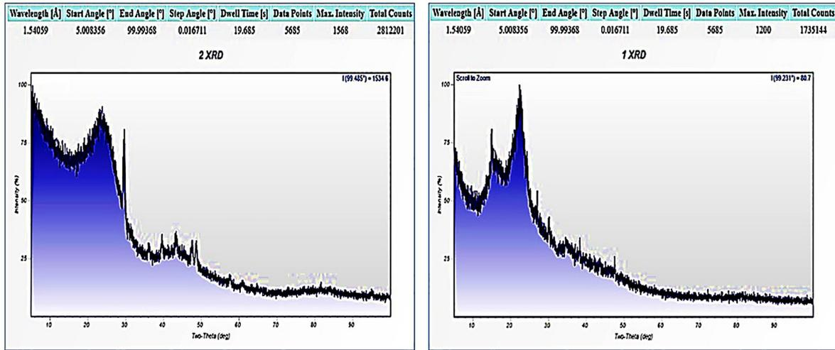
Figure 15: XRD images of (a) RBAC and (b) RSAC concrete mix with superplasticizer.
