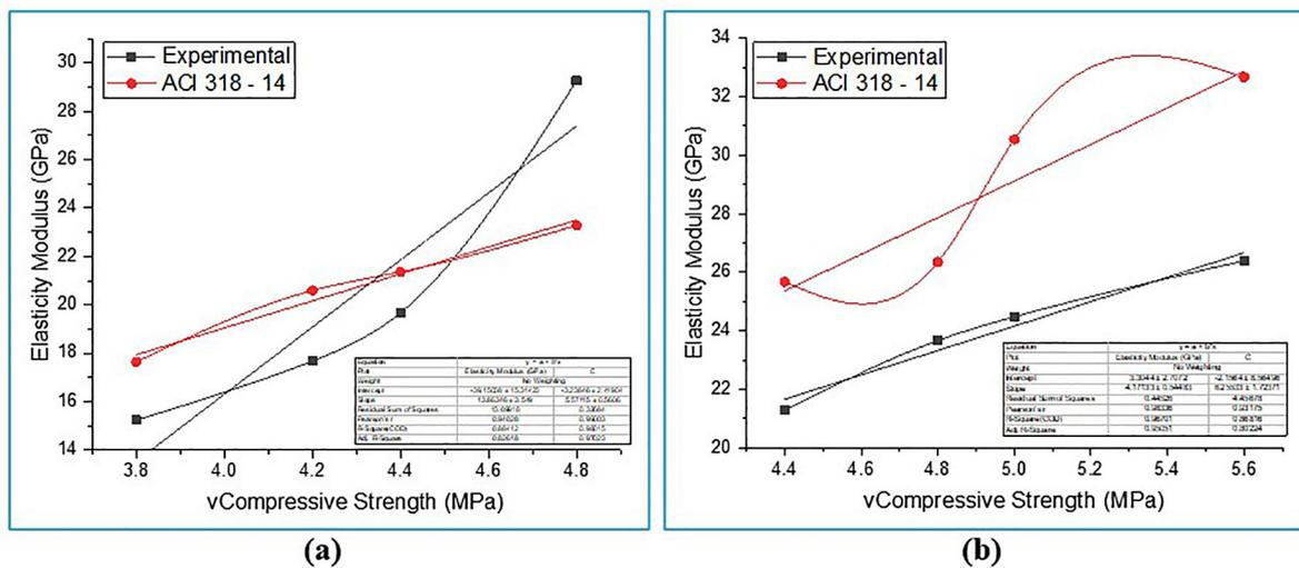
Figure 12: RBAC mixes – elasticity modulus and its relationship with/without superplasticizers.
