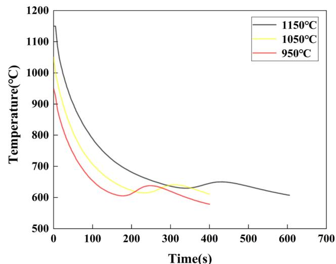
**Figure 3:** Cooling curves of the specimens after different austenitizing temperatures.
