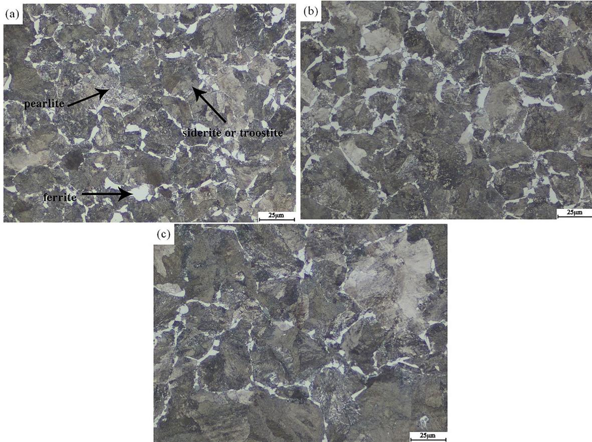
Figure 4: Microstructure of samples heated at different austenitizing temperatures (a) 950 °C; (b) 1050 °C; (c) 1150 °C.
