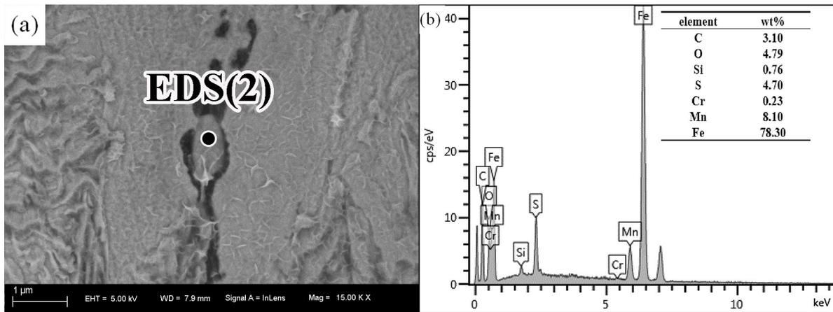
**Figure 10:** EDS analysis of precipitated phase near microcracks.
