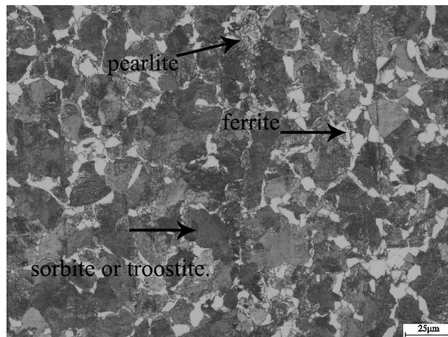
**Figure 1:** Original microstructure of experimental steel.
