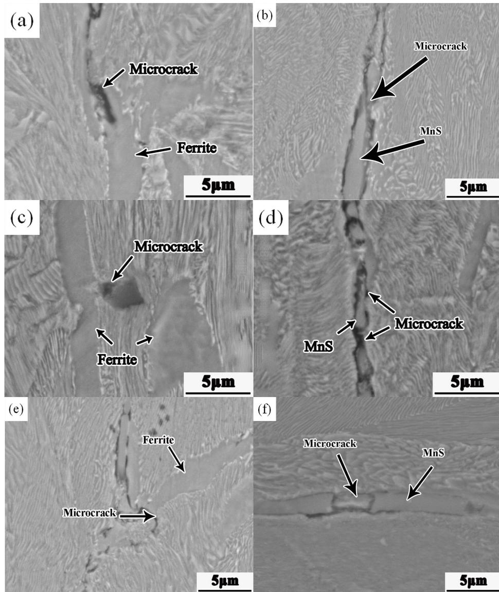
Figure 9: Microstructure near fracture of tensile specimens heated at different austenitizing temperatures (a)(b) 950 °C; (c)(d) 1050 °C; (e)(f) 1150 °C.
