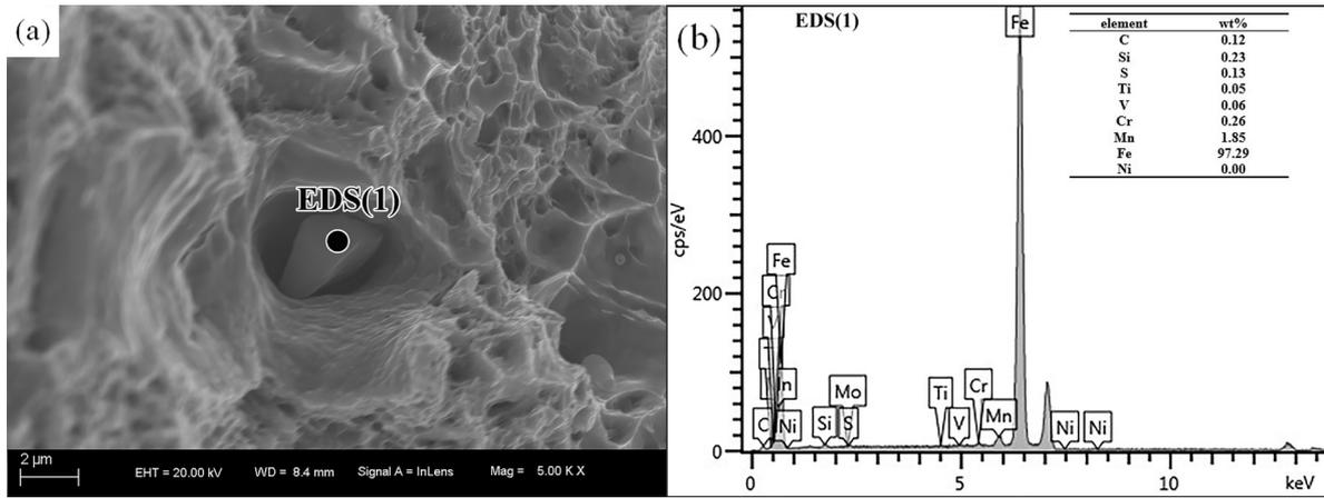
Figure 8: EDS analysis of particles at the bottom of dimples.
