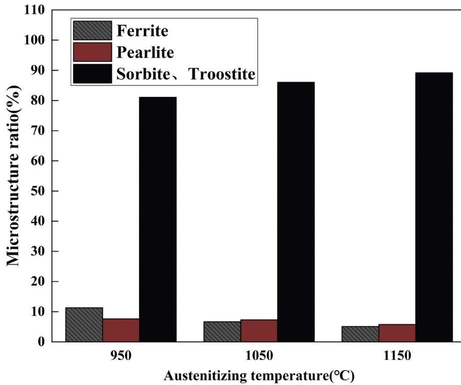
Figure 5: Microstructure percentage of the specimens after austenitizing at different temperatures.
