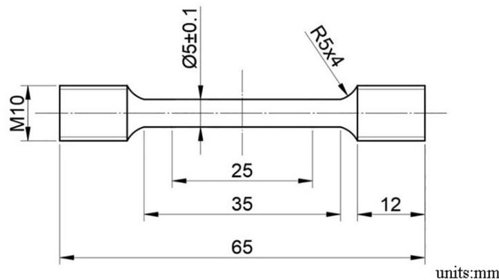
**Figure 2:** Diagram of tensile specimen.
