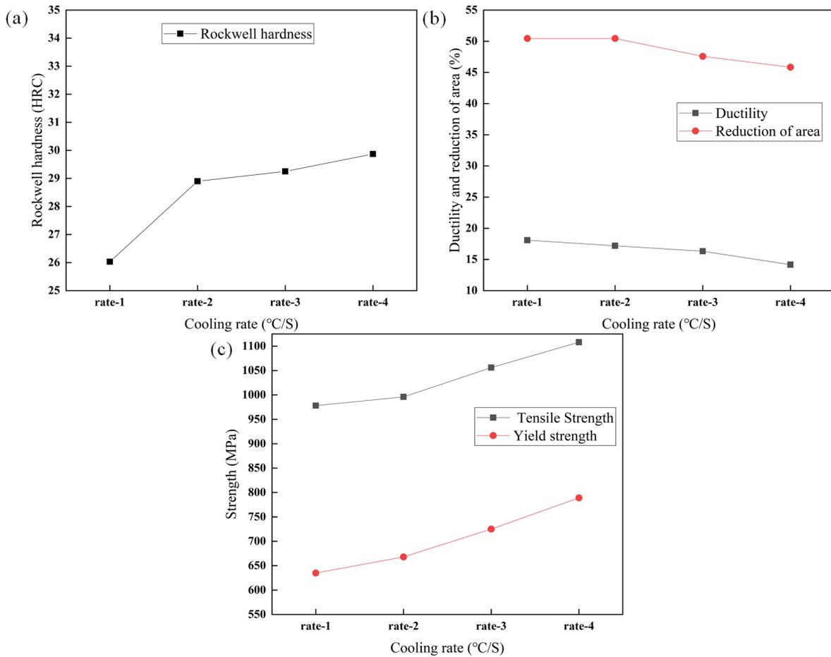
Figure 14: Mechanical properties of the specimens after cooling with different rates (a) rockwell hardness; (b) ductility and reduction of the area; (c) strength.
