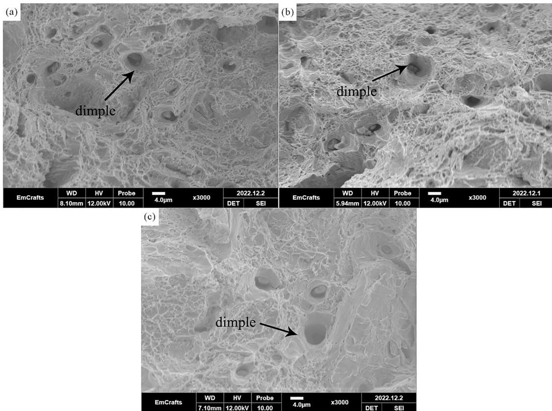
**Figure 7:** Fracture morphology of tensile specimens heated at different austenitizing temperatures (a) 950 °C; (b) 1050 °C; (c) 1150 °C.
