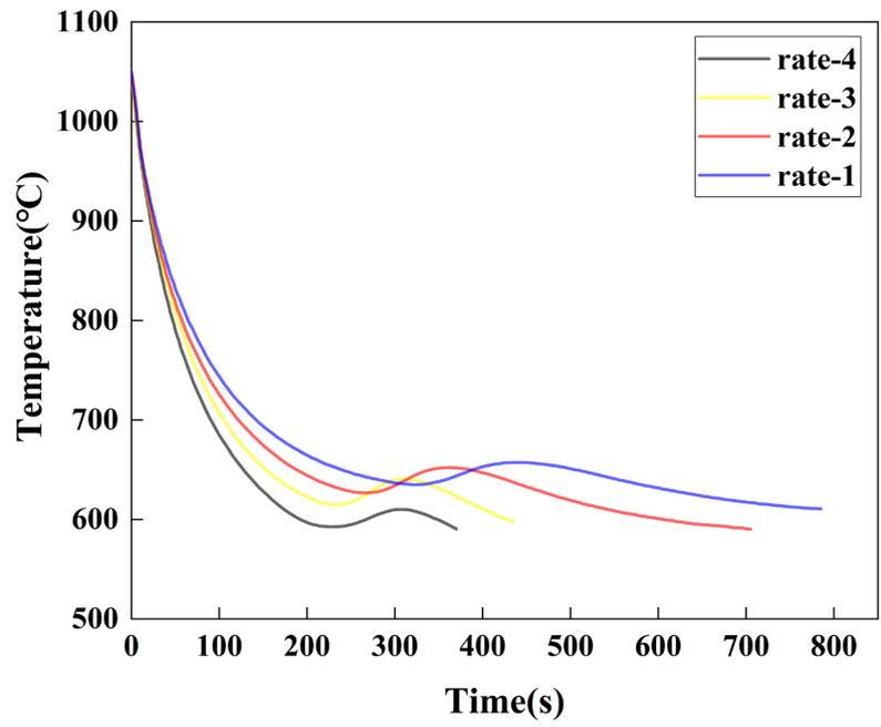
**Figure 11:** Cooling curves of the specimens after austenitizing with different cooling rates.
