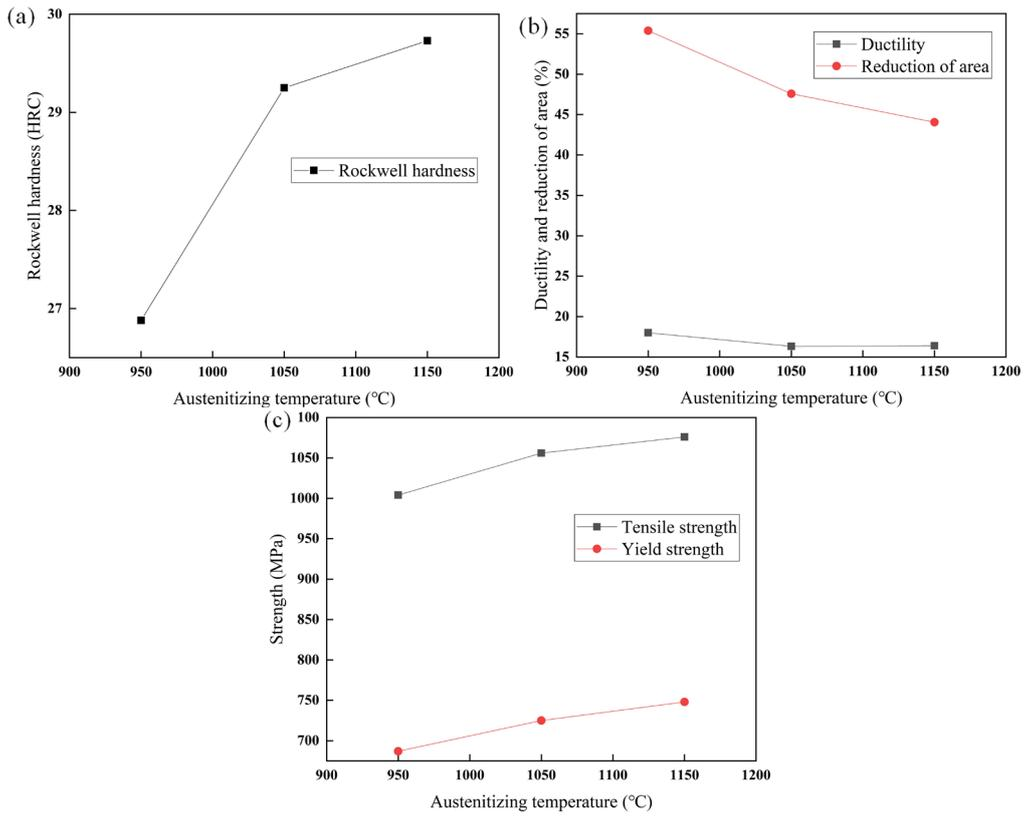
**Figure 6:** Mechanical properties of the specimens after austenitizing at different temperatures (a) rockwell hardness; (b) ductility and reduction of the area; (c) strength.
