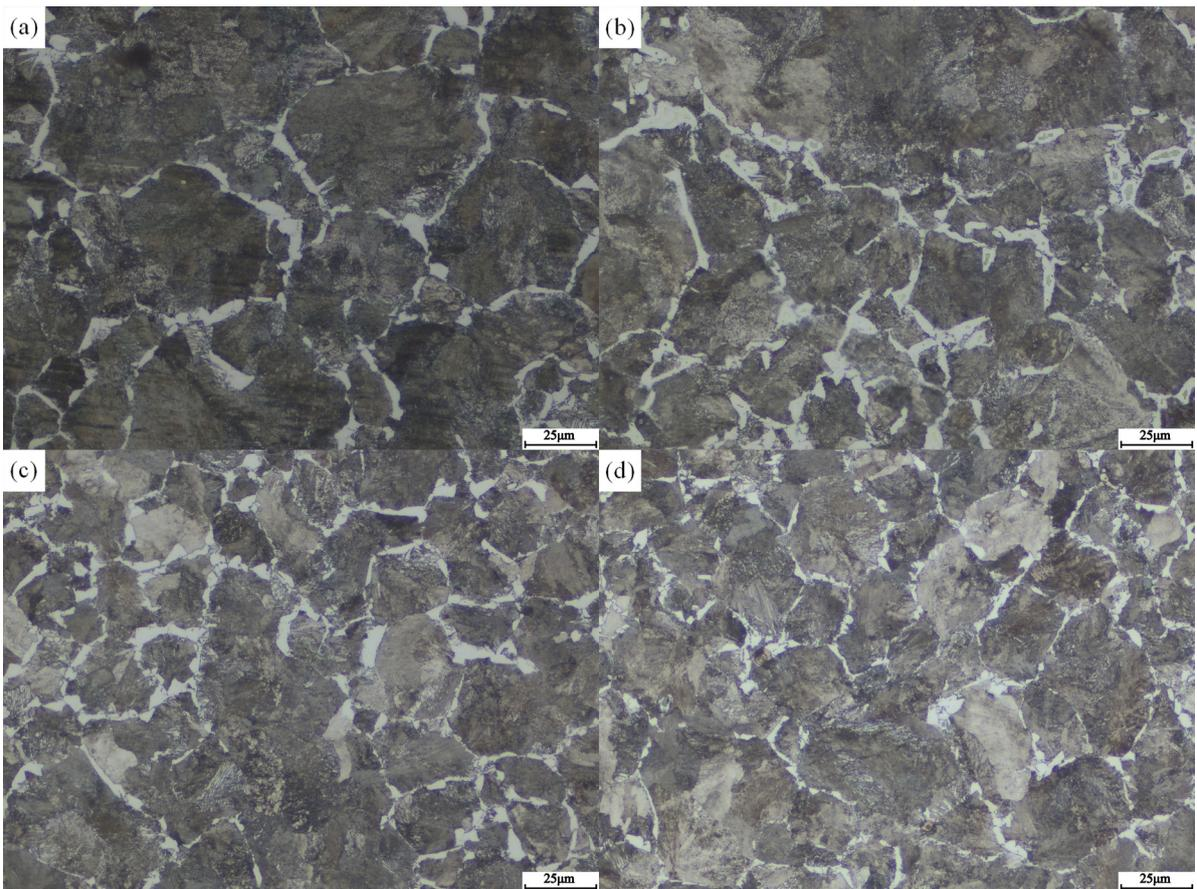
**Figure 12:** Microstructure of samples cooled at different cooling rates (a) rate-1; (b) rate-2; (c) rate-3; (d) rate-4.
