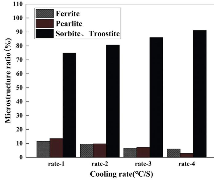
Figure 13: Microstructure percentage of the specimens after cooling with different rates.
