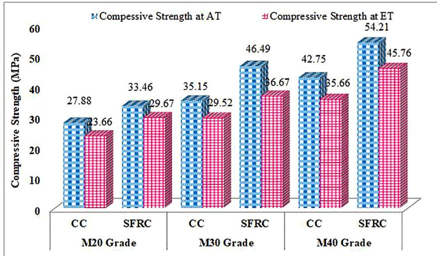
Figure 4: Compression strength of concrete at ambient and elevated temperatures.
