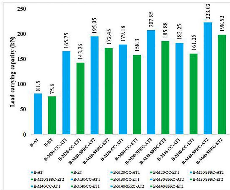
Figure 7: Load-carrying capacity of the CFST rectangular beam (ambient & elevated temperatures).
