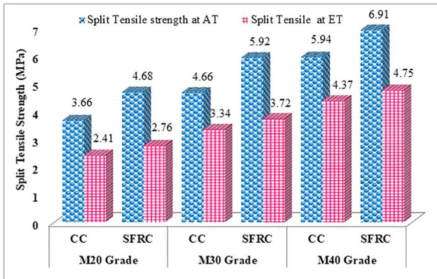
Figure 5: Split tensile strength of concrete at ambient and elevated temperatures.
