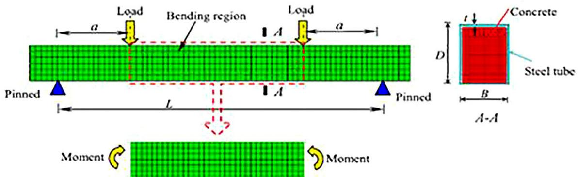
Figure 3: Boundary and mesh conditions.
