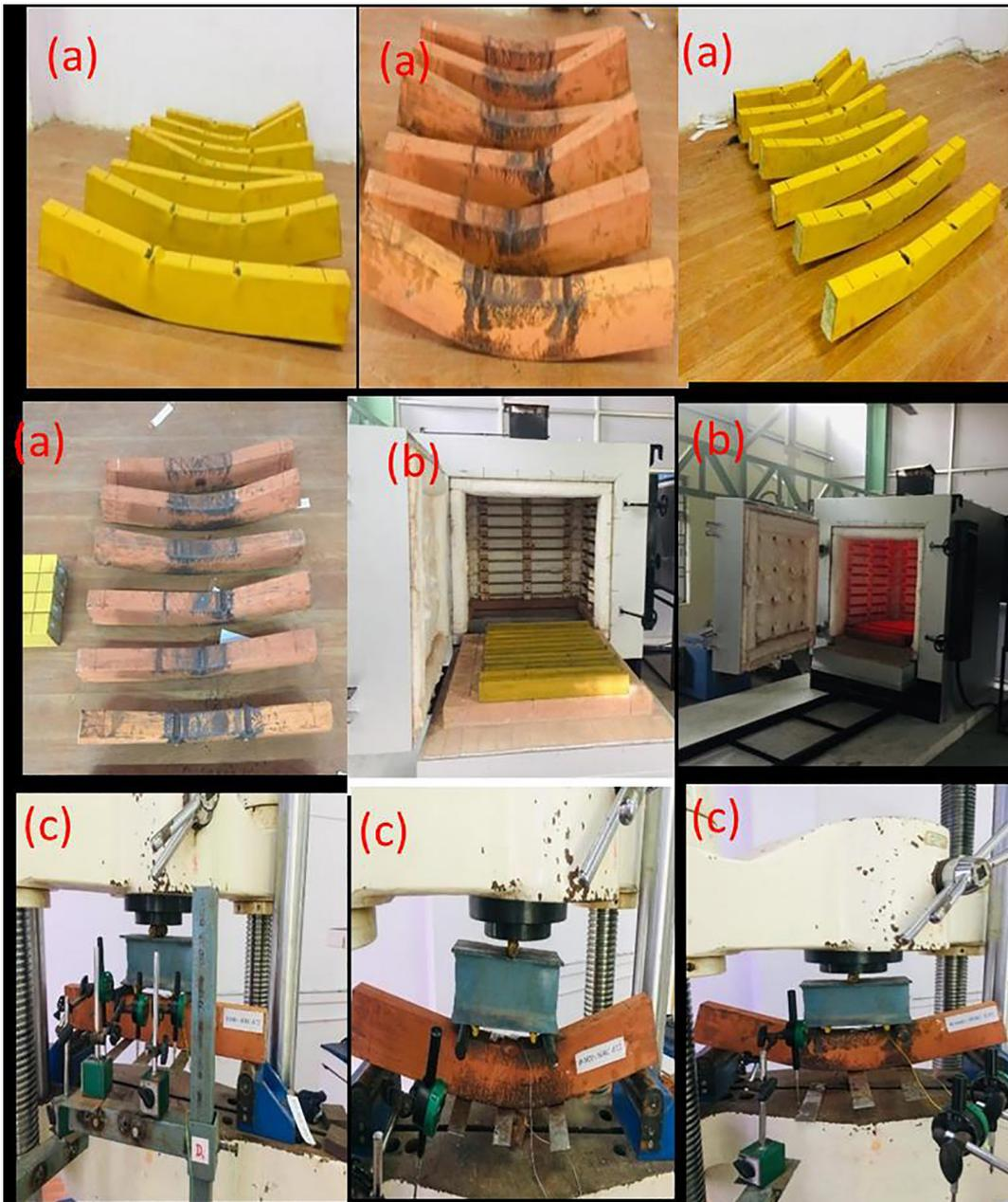
Figure 13: (a) CFST tested samples (b) elevated temperature (c) failure of the beams (ambient and elevated temperature).
