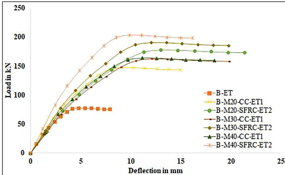
Figure 10: Load vs. deflection at elevated temperature in beams.
