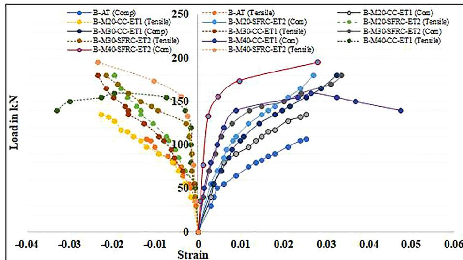
Figure 12: Load vs. strain at elevated temperature in beams.
