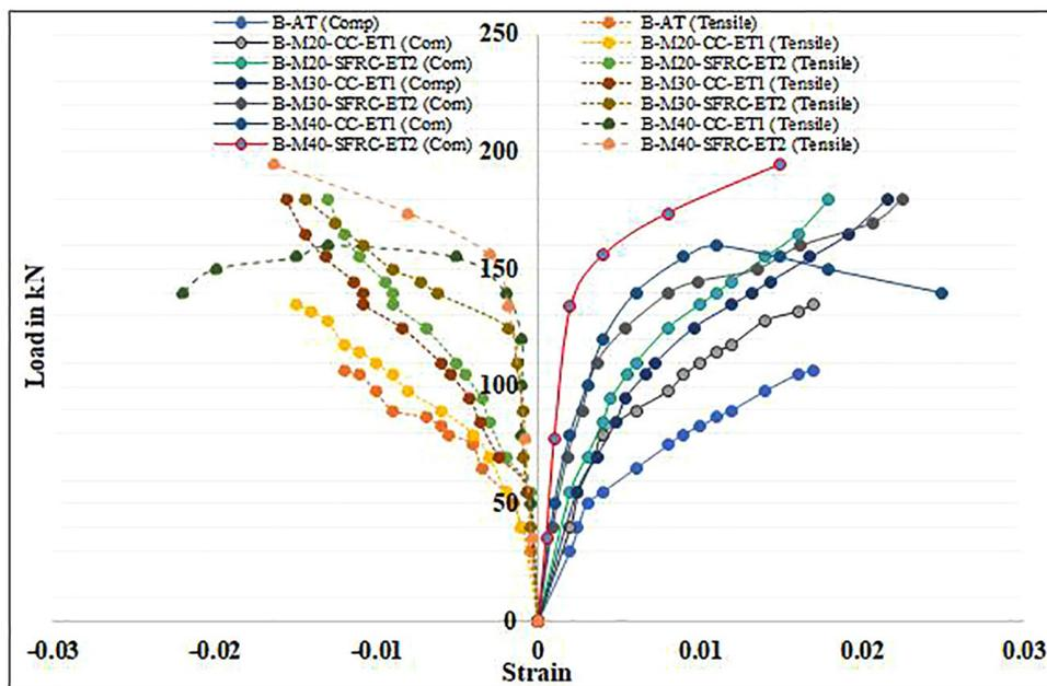
Figure 11: Load vs. strain at ambient temperature in beams.
