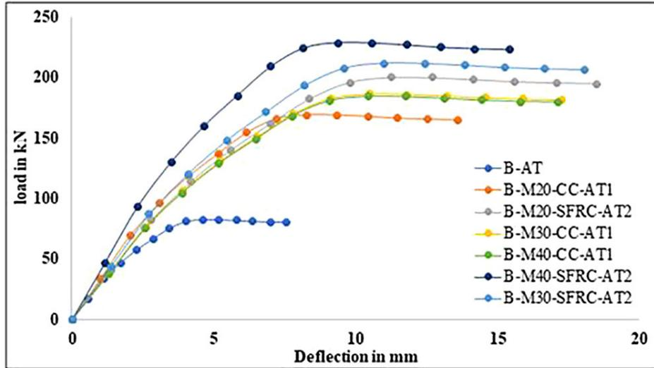
Figure 9: Load vs. deflection at ambient temperature in beams.
