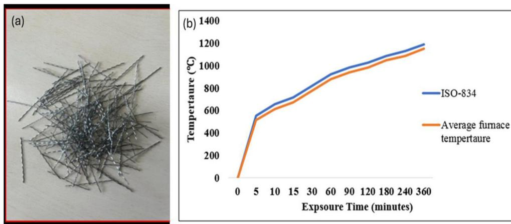
**Figure 1:** (a) Steel fibers; (b) furnace temperature vs. ISO-834.
