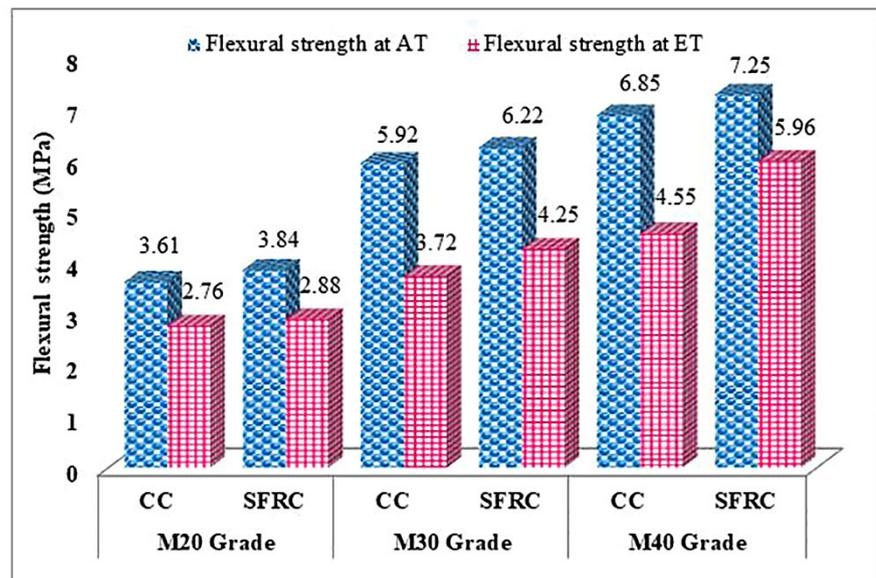
Figure 6: Flexural tensile strength of concrete at ambient and elevated temperatures.
