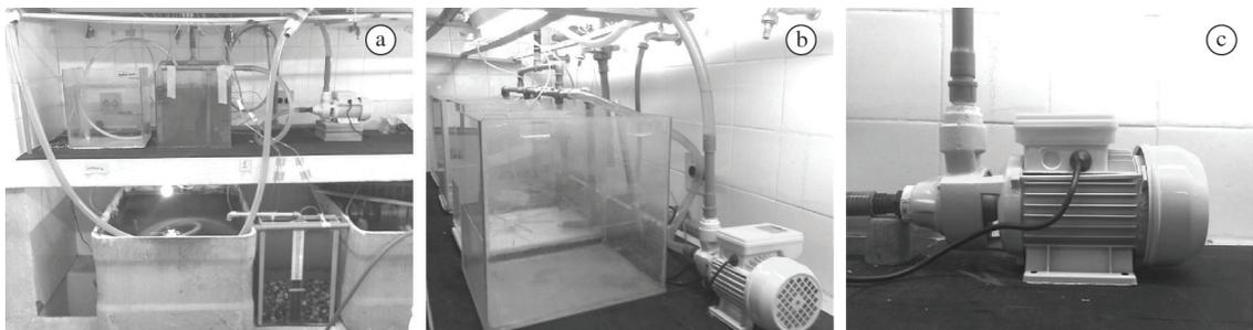
**Figure 1.** Mill developed for closed circulation of water and maintenance of the turbidity of the experiment: (a) hydraulic assembly; (b) detail of pipe connections; (c) pump used in the experiment.
