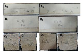
**Figure 11:** Decreasing dimensions (A, C) and closing (B, D) in checks (0: Before, 1: After).
