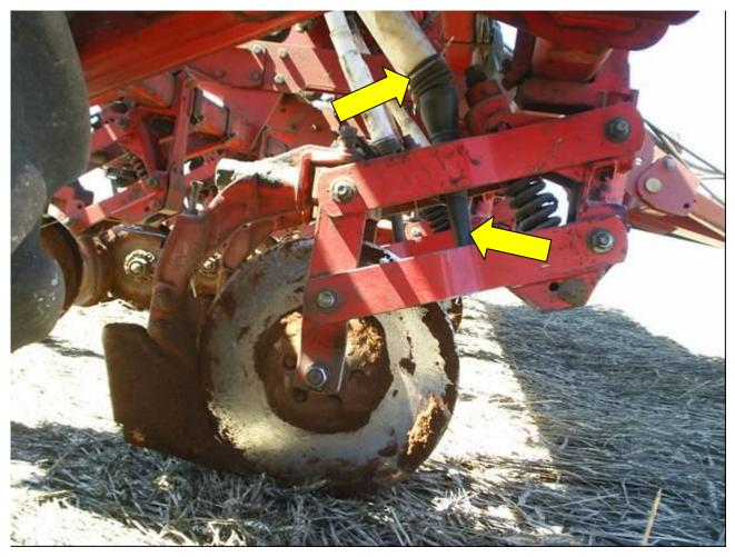
FIGURE 2. Sower fertilize with fertilizer distribution in front of the cutting disk tillage under the mulch in the region of Campos Gerais - PR.
