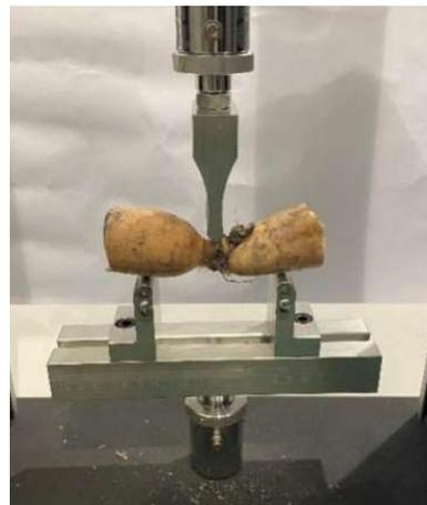
FIGURE 6. Lotus root bending test.
