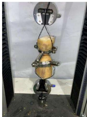
FIGURE 7. Lotus root tensile test.
