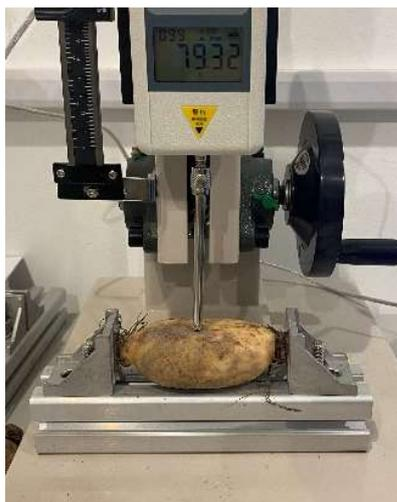
FIGURE 4. Lotus root body compression test.
