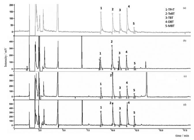
Figure 1. Chromatograms (GC-PFPD) for BTs spiked into the investigated matrices: (a) solvent (hexane), (b) sediment, (c) liver and (d) gills.
