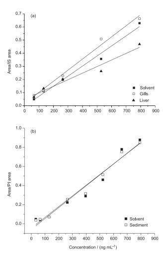
Figure 2. Calibration curves for TBT in the matrix effect study: (a) fish tissue and (b) sediment.
