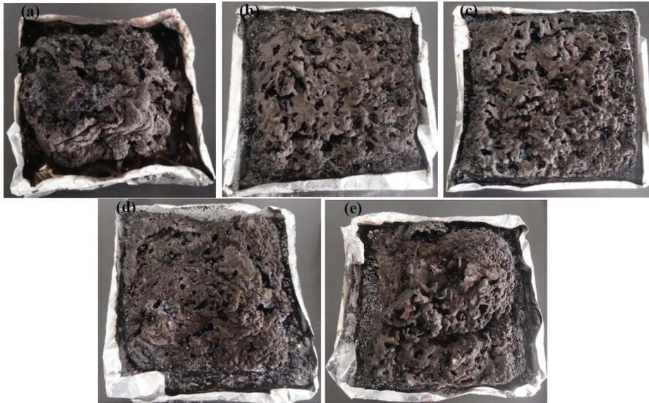
**Figure 6.** Morphology photographs of the char residuals of experimental materials tested by cone calorimeter testing. (a) PVC0, (b) PVC1, (c) PVC2, (d) PVC3, (e) PVC4.
