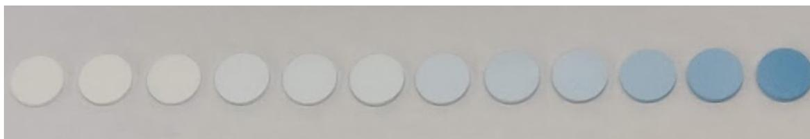
**Figure 1.** Samples after thermal treatment. From left to right, the  $\text{Co}^{2+}$  concentration increases at the following order: 0.003, 0.004, 0.03, 0.05, 0.08, 0.1, 0.2, 0.3, 0.5, 1, 2 and 5 at. mol% of  $\text{Co}^{2+}$ .
