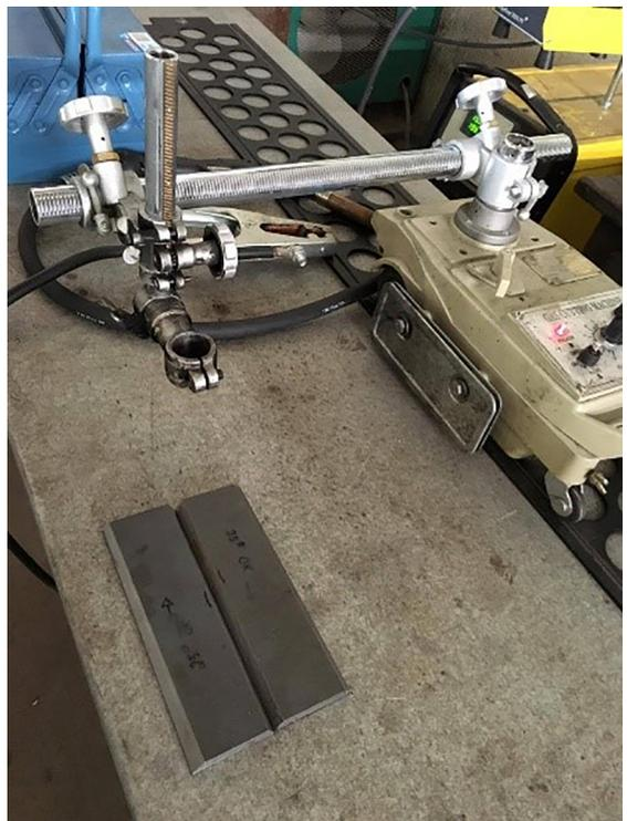
Figure 3. Gas-cutting machine.
