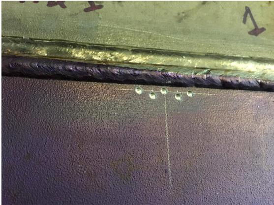
**Figure 4.** Sample drilled holes.
