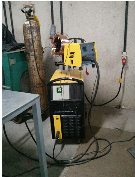
Figure 2. MAG welding semiautomatic machine.
