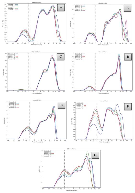
Figure 2. Particle size distribution over time (1.5; 3.0; 4.5; 6.0 e 7.5 minutes)
