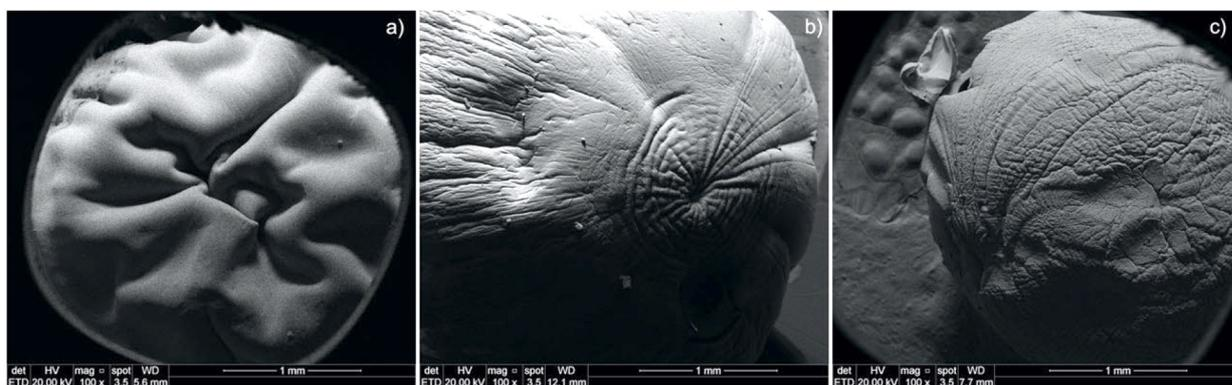
**Figure 6.** SEM images of the spheres surface: (a) silicate/alginate; (b) *Ludox/alginate*; (c) silicate/*Ludox/alginate*
