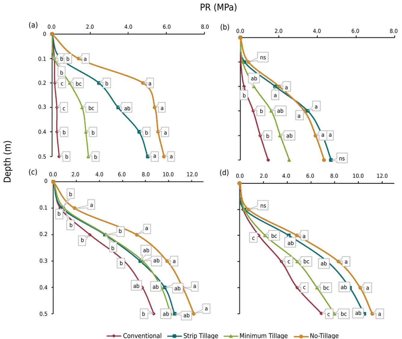
**Figure 2.** Soil penetration resistance (PR) for the following measurement dates: (a) 10/3/19, (b) 12/18/19, (c) 1/30/20, (d) 3/10/20, with the average comparing the soil management in each layer (depth). ns: not significant by the Tukey (5 %).
