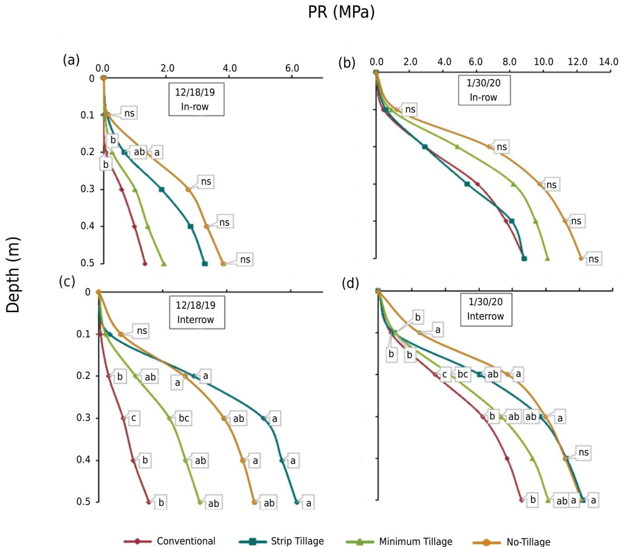
**Figure 3.** Soil penetration resistance (PR) at different dates and measurement positions (a) 12/18/19 in-row, (c) 12/18/19 interrow, (b) 1/30/20 in-row, (d) 1/30/20 interrow, means comparing the soil management in each soil layer (depth). ns: not significant by the Tukey (5 %).
