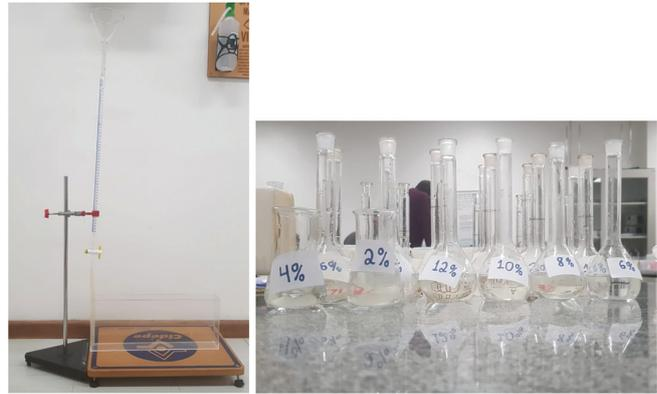
**Figure 7:** Apparatus for (a) the concentration gradient, and (b) graduated sugar solutions.
