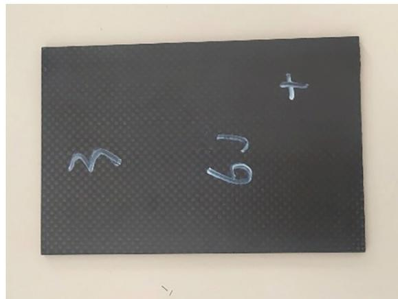
Figure 13: The CFRP laminates.
